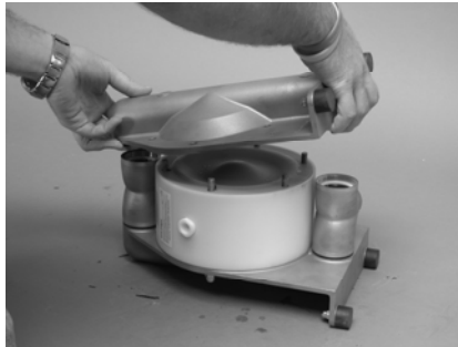
Remove side housing [1] and suction/discharge ports [2].
