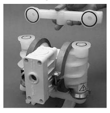
Remove discharge manifold. It is now possible to inspect the outboard o- rings.
