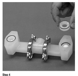
Remove the discharge valve balls, seats and o-rings from the discharge manifold and inspect for nicks, gouges, chemical attack or abrasive wear. Replace worn parts with genuine Wilden parts for reliable performance. PTFE o-rings should be replaced when reassembled.
