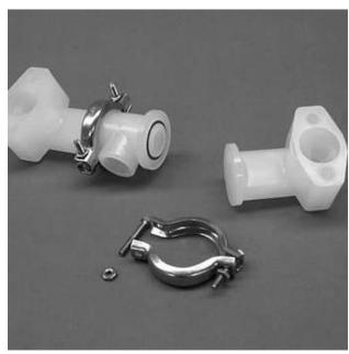
**Step 7**Inspect o-rings for wear or damage and replace if necessary.
