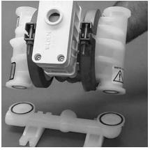
Lift center section off of the inlet mani- fold. It is now possible to inspect the outboard orings on the inlet manifold.
