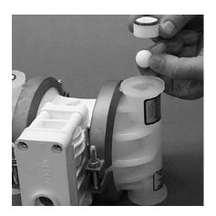
Place center section upside-down on a flat surface. Remove the o-ring, seat and valve ball from the bottom of the water chamber. It is now possible to inspect these parts. If swelling, cracking or other damage is apparent these parts must be replaced.
