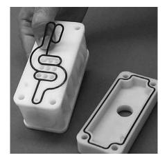
**Step 3**Lift away air valve assembly and remove air valve gasket for inspection. Replace if necessary.
