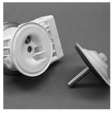
To remove the remaining diaphragm assembly from the shaft, secure shaft with soft jaws (a vise fitted with plywood or other suitable material) to ensure shaft is not nicked, scratched, or gouged. Using an adjustable wrench, remove diaphragm assembly from shaft. Inspect all parts for wear and replace with genuine Wilden parts if necessary.
