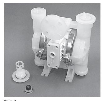
**Step 4**Remove the top liquid retainer and retainer O-rings, discharge valve balls, seats and valve seat O-rings from the liquid chamber and inspect for nicks, gouges, chemical attack or abrasive wear. Replace worn parts with genuine Wilden parts for reliable performance.
