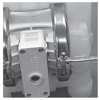
**Step 7**With a 1/2" box wrench, loosen the large clamp bands that secure the liquid chambers to the center section.
