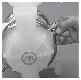
**Step 8**Rotate the clamp bands so that they can be removed.
