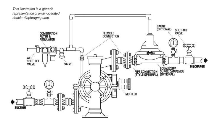
NOTE: In the event of a power failure, the shut-off valve should be closed, if the restarting of the pump is not desirable once power isregained.
