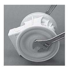
**Step 11**Using two 1" sockets, remove diaphragm assembly from center section assembly.
