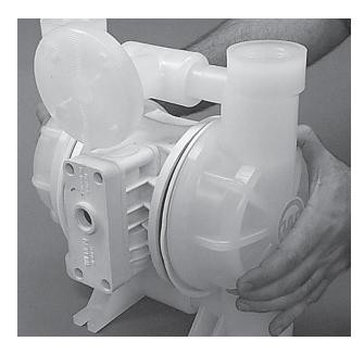
**Step 9**After clamp bands are removed, pull liquid chambers apart.
