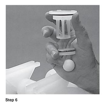
Remove the bottom liquid retainer and retainer O-rings, discharge valve balls, seats and valve seat O-rings from the liquid chamber and inspect for nicks, gouges, chemical attack or abrasive wear. Replace worn parts with genuine Wilden parts for reliable performance.
