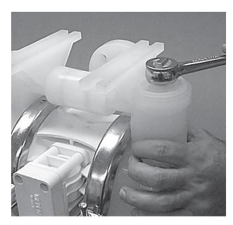
**Step 5**Using a 1/2" socket driver, loosen the bottom retainers.
