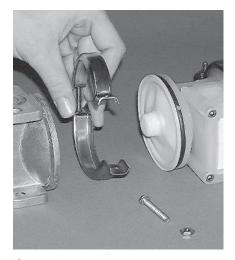
**Step 7** After clamp bands are removed, pull chambers away from center section.
