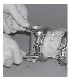
Step 6 Loosen clamp band with 5/16" socket and 3/8" wrench. Remove screw and nut.
