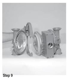
Pull liquid chamber away from the center section to expose diaphragm and outer piston. Remove other side of the liquid chamber from center section.
