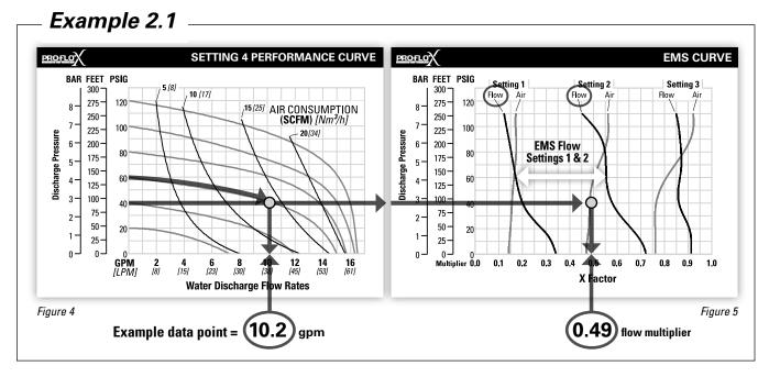
This is an example showing how to determine the inlet air pressure and the EMS setting for your Pro-Flo X™ pump to optimize the pump for a specific application. For this example we will be using an application requirement of 18.9 lpm (5 gpm) flow rate against 2.8 bar (40 psig) discharge pressure. This example will illustrate how to calculate the air consumption that could be expected at this operational point.
