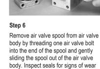
and replace entire assembly if necessary. Use caution when handling air valve spool to prevent damaging seals.
