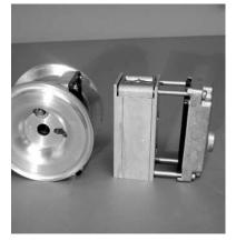
Step 2 Remove the air valve and muffler plate from the center section.
