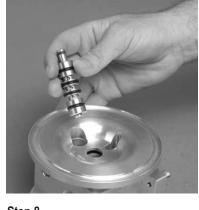
Step 8 Remove pilot spool assembly from center section.
