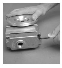
Step 1 Using a 3/16" hex head wrench, loosen the air valve bolts.
